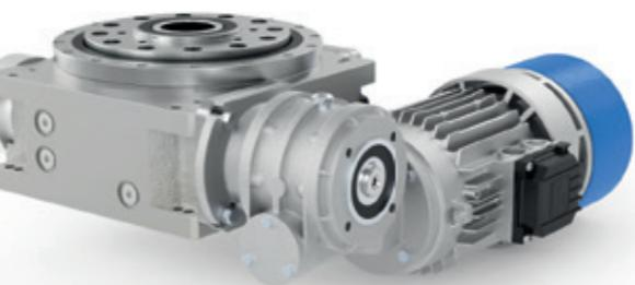
The **TRP** Series are designed for accurate and repeatable rotary indexing applications this heavy duty design provides a precision barrel cam set, solid cam follower technology and oversized cross roller bearing to support the output turret.
